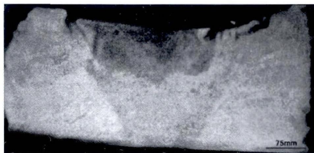
图 1 工艺改进前 H13 钢锭头部低部组织形貌 Fig. 1 Morphology of macrostructure of steel H13 ingot top before process improvement
